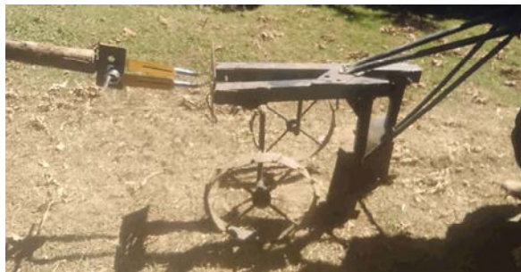
Fig. 18: Multiple mouldboard plough spring dynamometer setup [Photo by the authors]
