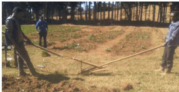
Fig. 19: Ard plough spring dynamometer setup [Photo by the authors]
