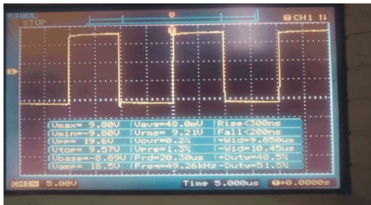
Fig. 23: Pulse generated using Arduino for a duty ratio of 0.5
