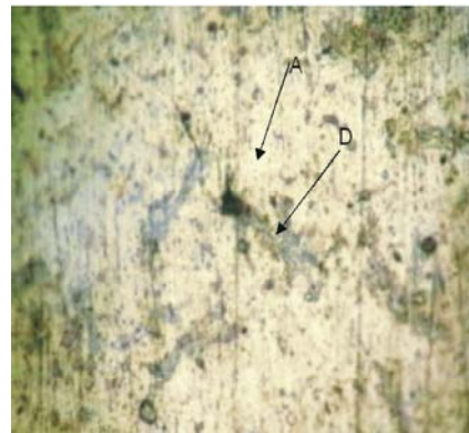
Fig. 6: Microstructure of weld metal at 95A. Magnification: x200
