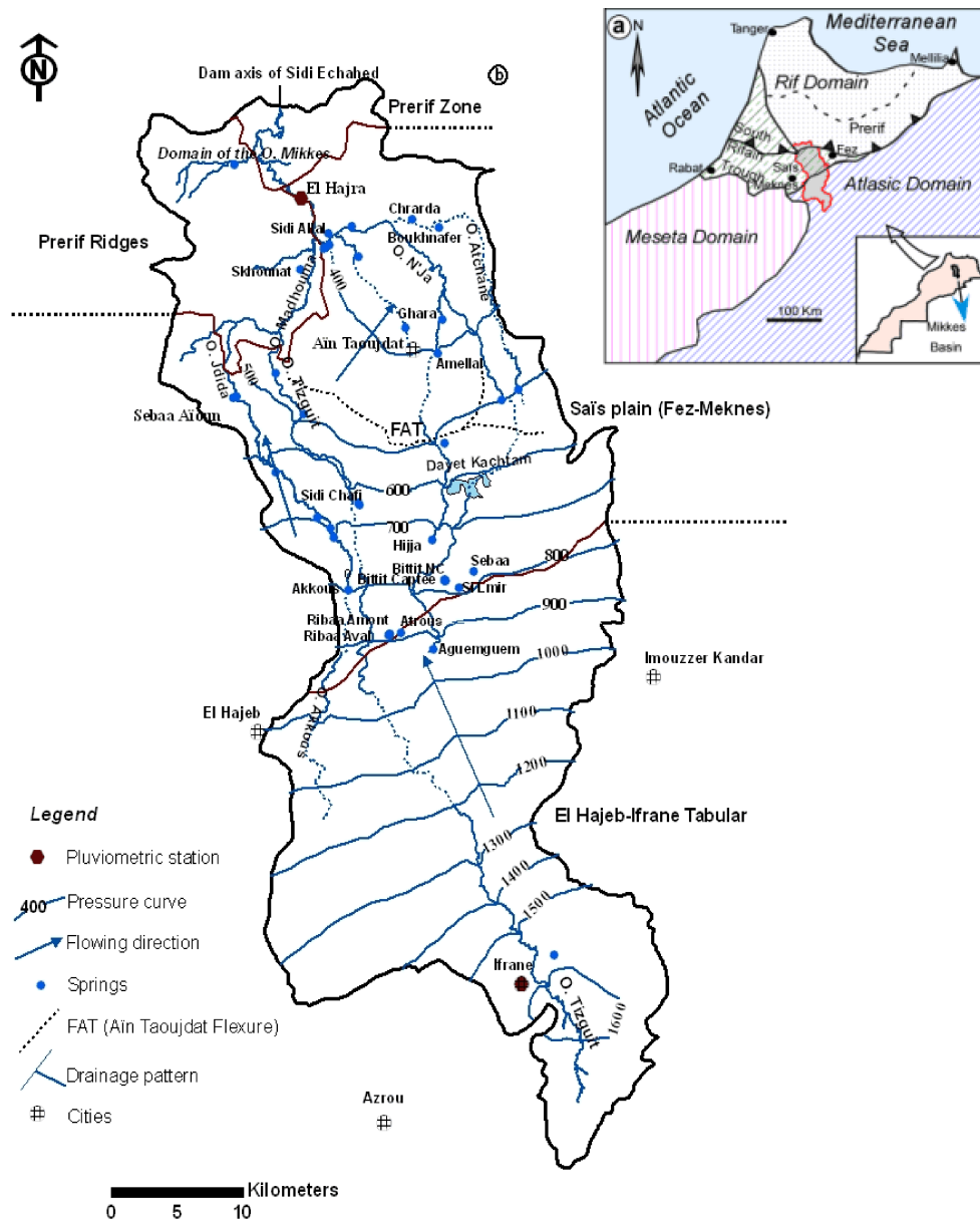
Fig. 1: a. Location of the Mikkes basin, b. Drainage pattern and piezometric map 2009 of the free-water table Mikkes (taken from the topographic map 1/100000, geology division, Rabat, Morocco, 1943)
