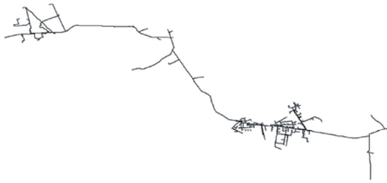
Fig 1: Single-line diagram of actual power network of Kosar feeder of Kerman Province in Cymedist
