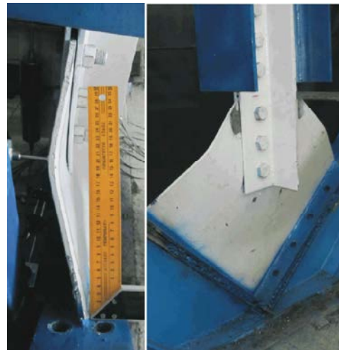
Fig. 5: Buckling of the model
