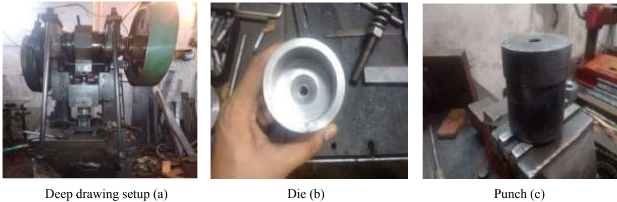
Fig 1: Deep drawing setup with available die & punch
