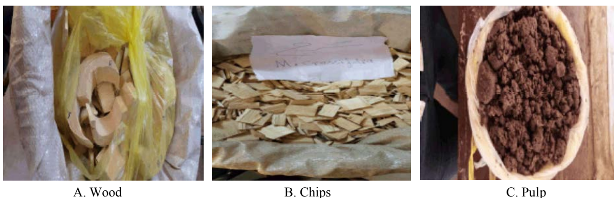
Fig 3. Steps of cooking of Maerua crassifolia (Sarah) with Soda-AQ pulping
