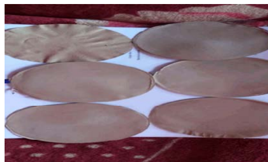
Fig. 4: Prepared hand sheets from pulp of Maerua crassifolia (Sarah) wood for physical properties
