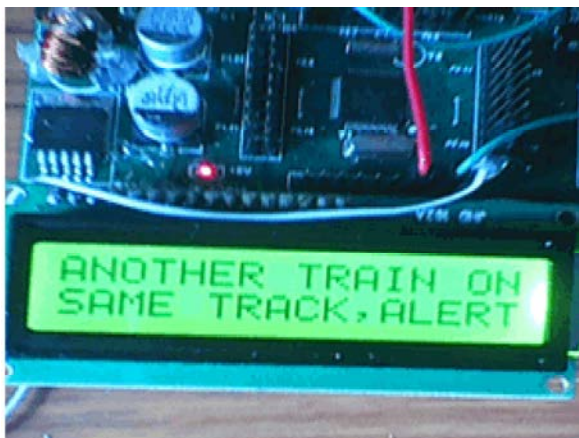
Fig. 6: Display of Alert Message When Two Trains Are in Same Track
