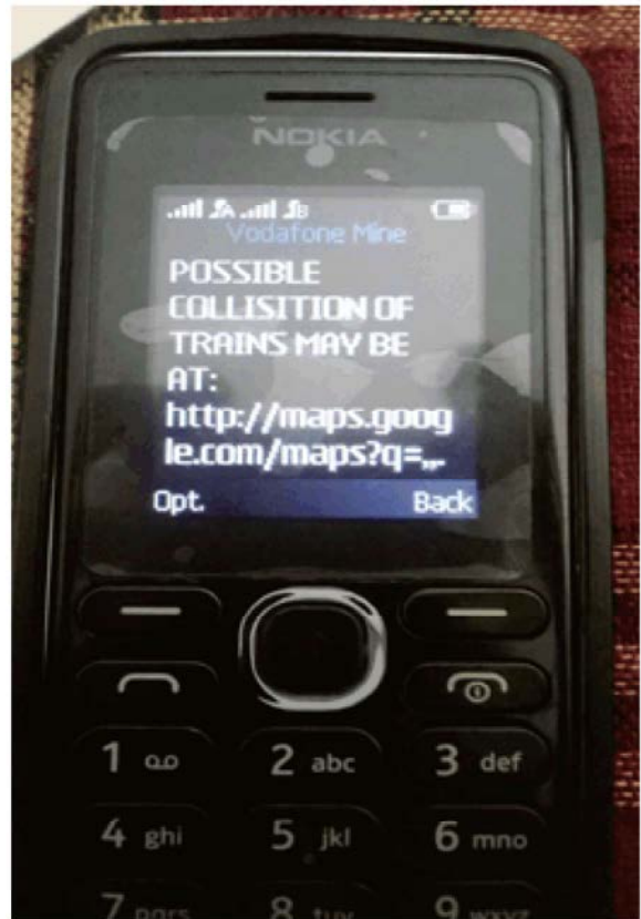
Fig. 8: Display of Message Alert When Two Trains Come to Same Track to Station Master.
