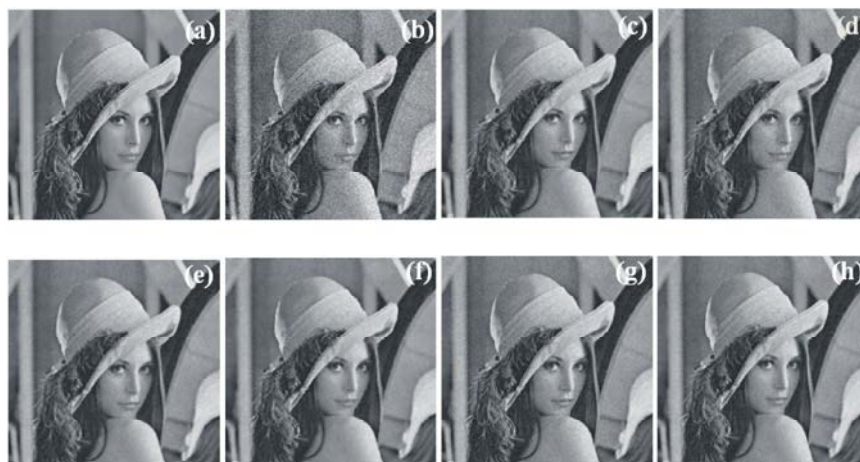
Fig. 8: Performance of Various Filters for Lena Image with AWGN \sigma_n = 15 (a) Original image (b) Noisy image (c) – (h): Results of various filtering schemes (c) Mean (d) ATM (e) Wiener (f) Lee (g) Bilateral (h) Proposed filter
