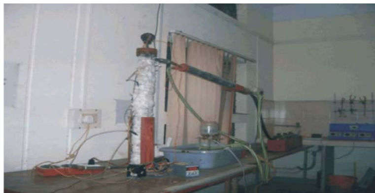
Fig. 2: Pyrolysis set up for bio-oil production
