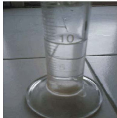
Fig. 3: Disitegtaion Using Measuring Cylinder Method
