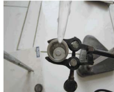
Fig. 2: Disitegtaion Using Basket Method
