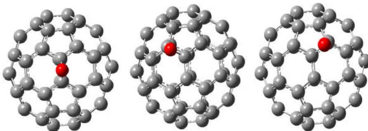
Fig. 1: Schematic view of the C 60 O configurations corresponding to the [6, 6], transition state and [5,6] position. Oxygen atoms are in red.
