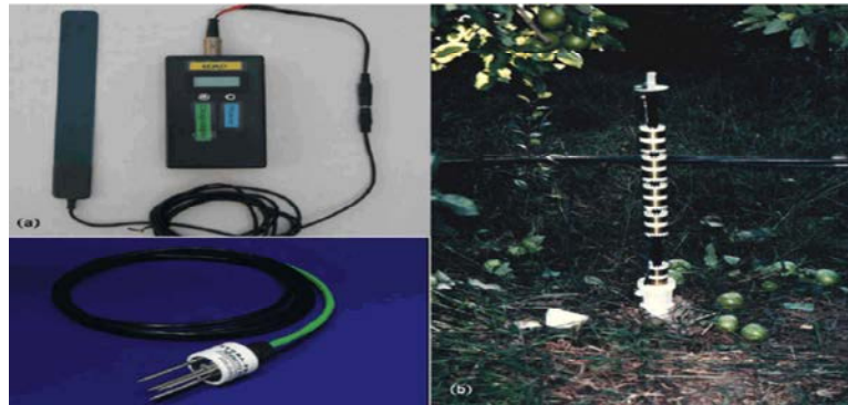
Fig. 3: FD probes: a) Capacitance (plates imbedded in a silicon board); b) Capacitance (rods); and c) FDR (rings)
