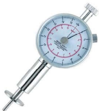
Fig. 1: Handheld fruit penetrometer or fruit firmness tester
