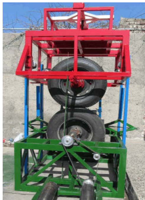
Fig 2: Tire deflection test apparatus
