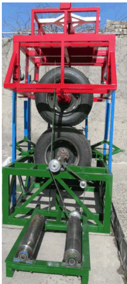
Fig. 3: Tire contact length measurement apparatus
