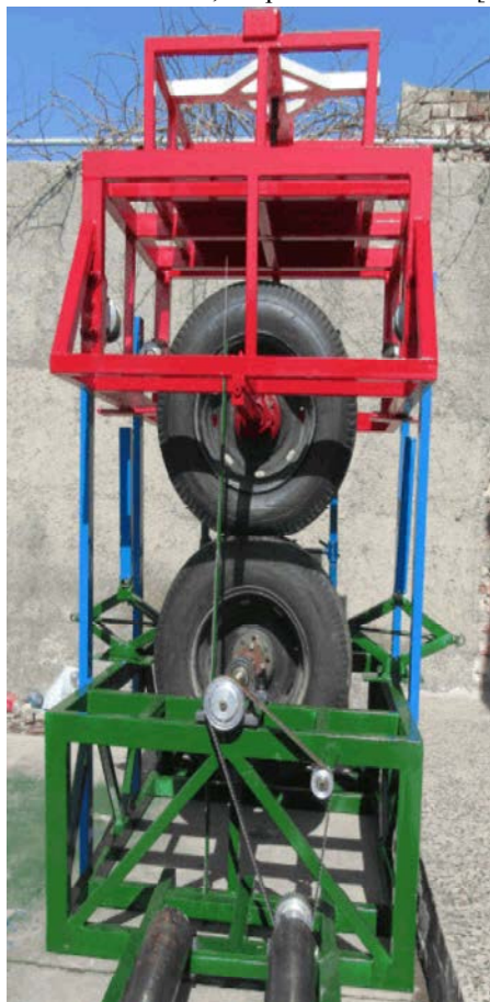
Fig. 2: Tire deflection test apparatus
