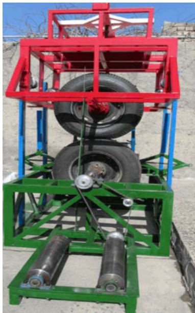
Fig. 3: Tire contact length measurement apparatus
