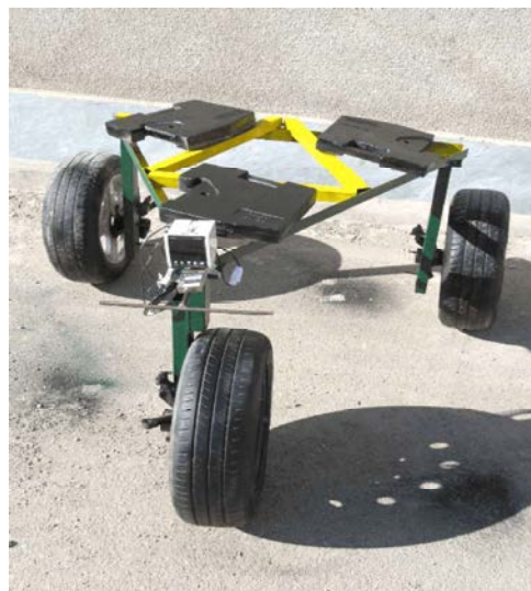
Fig. 1: The tire rolling resistance test apparatus, linkages, weights, load cell and data logger
