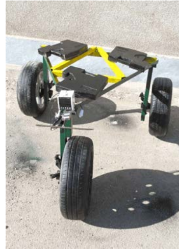
Fig. 1: The tire rolling resistance test apparatus, linkages, weights, load cell and data logger
