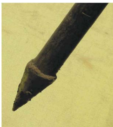
Fig. 3: Small cone size (diameter: 12.83 mm; area: 130 mm 2 ; angle: 30°)
