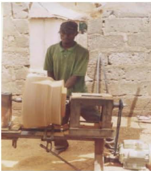
Plate 1: An operator processing P. africana stem into mortar
