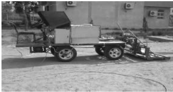
Fig. 2: The ESCALAD trolley: to the right the neutron detectors are seen, mounted on a positioning system. To the left is the driver seat where the speed control, steering and data inspection are located.
