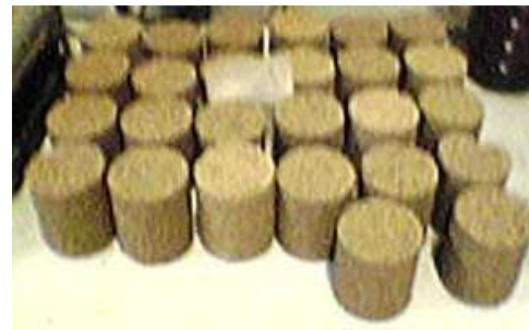
Fig. 1: Samples of green compressive strength, permeability and shatter index test specimens
