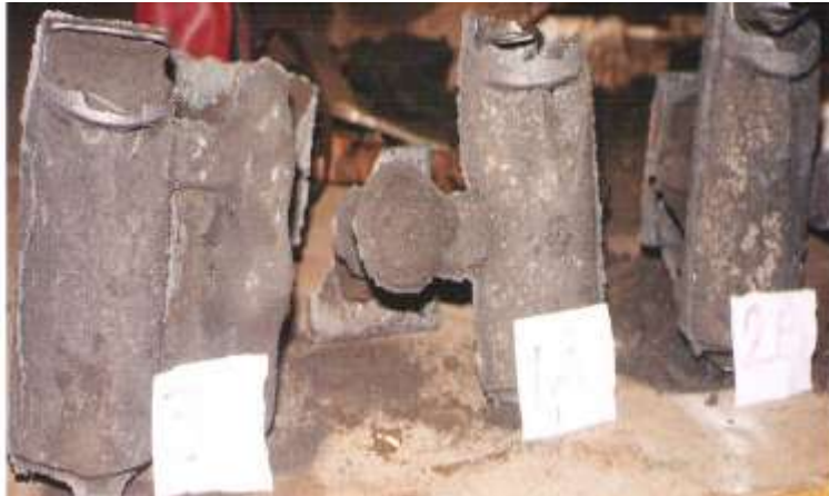
Plate 3: Experimental castings as shaken out from the sand moulds
