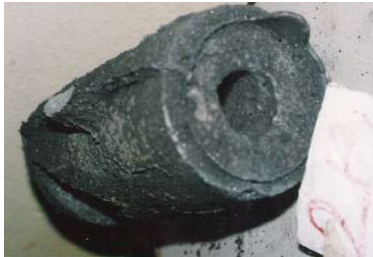
Plate 4: A typical casting revealing cavity created by a core bonded with kaolin/gum Arabic grade 4 composite.
