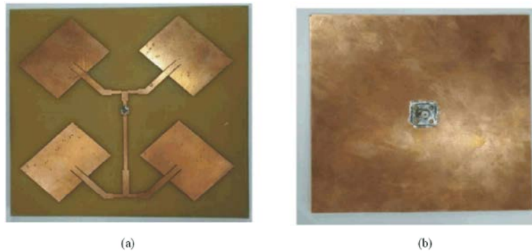
Fig. 8: Fabricated 2x2 patch antenna array (a) top view and (b) bottom view
