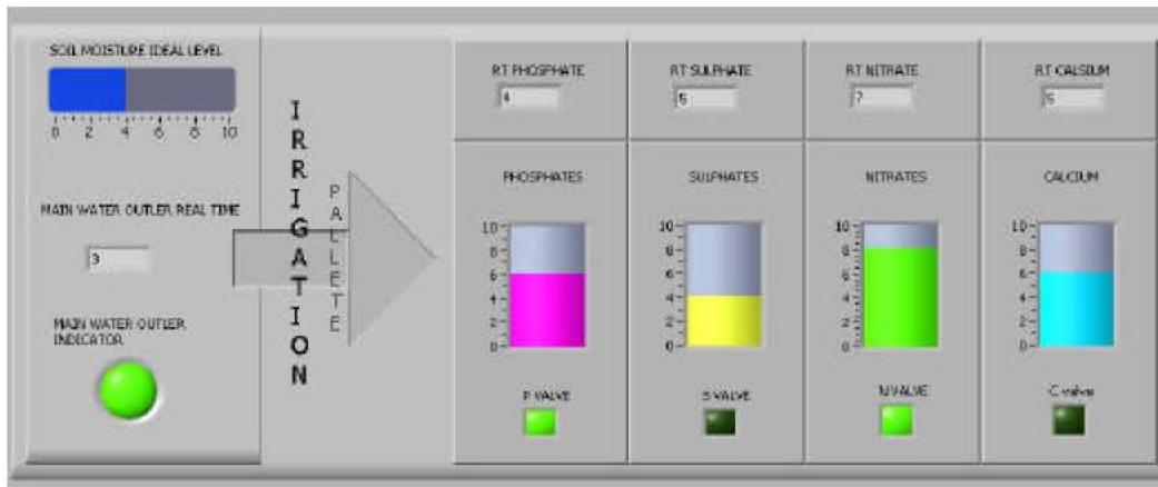
Fig. 3: Front panel of irrigation and fertilization subsystem
