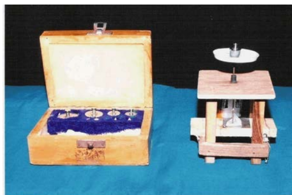
Fig. 2: Apparatus for investigation of hardness of carvediolol transdermal films.
