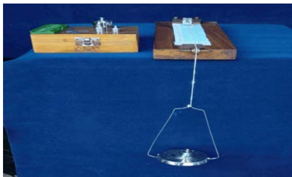
Fig. 1: Apparatus for testing of tensile strength.
