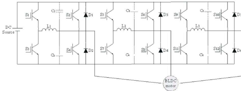
Fig. 3: Three phase resonant inverter
