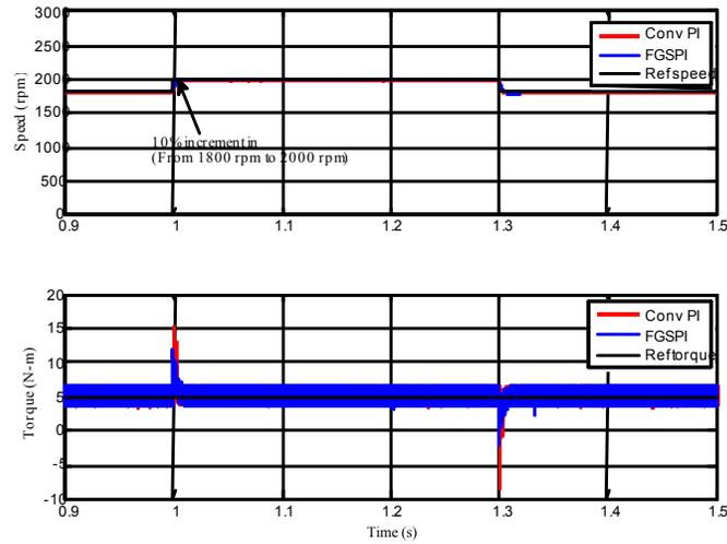
Fig. 15: Speed and torque responses of HEV system for change in speed ( $N=1800$  rpm up to 1 sec,  $T=5N\cdot m$ ;  $t=1 - 1.3$ sec,  $N=2000$  rpm,  $T=5N\cdot m$ ;  $t=1.3 - 1.5$ sec,  $N=1800$  rpm,  $T=5N\cdot m$ )
