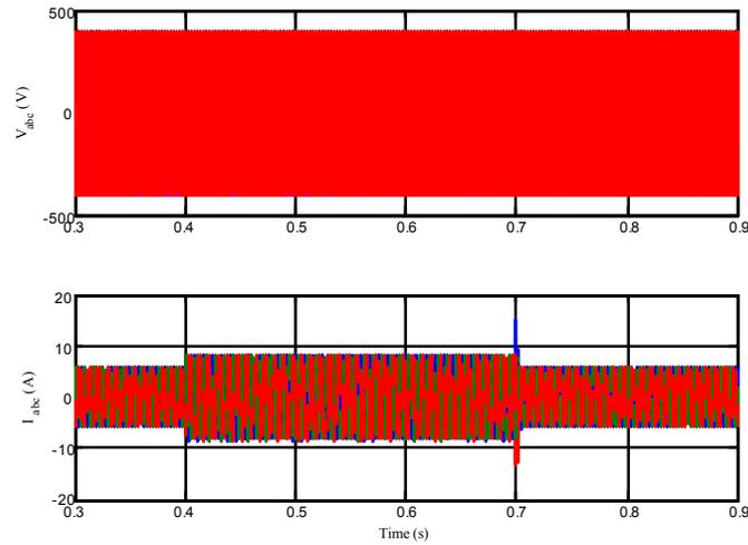
Fig. 14: Voltage and current responses of HEV system for change in speed (up to 0.4sec,  $N=1800$  rpm,  $T=5N\cdot m$ ;  $t=0.4 - 0.7$ sec,  $N=1600$  rpm,  $T=5N\cdot m$ ;  $t=0.7 - 1$ sec,  $N=1800$  rpm,  $T=5N\cdot m$ )
