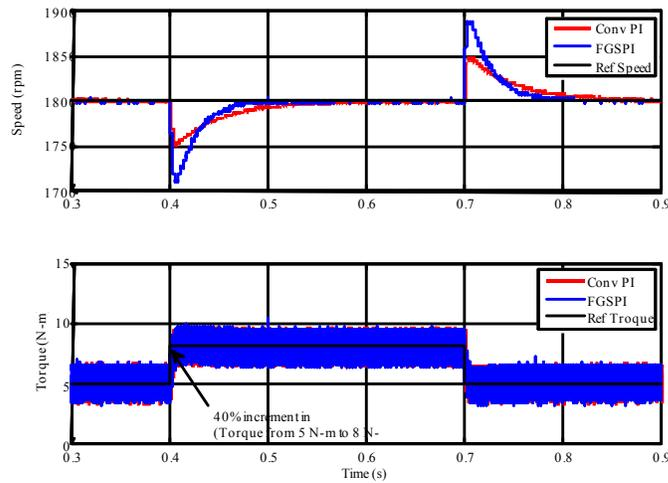
Fig. 17: Speed and torque responses of HEV system for change in load (up to 0.4sec,  $T=5\text{N-m}$ ,  $N=1800\text{ rpm}$ ;  $t= 0.4 - 0.7\text{sec}$ ,  $T=8\text{ N-m}$ ,  $N=1800\text{ rpm}$ ;  $t= 0.7 - 1\text{sec}$ ,  $T=5\text{ N-m}$ ,  $N=1800\text{ rpm}$ )
