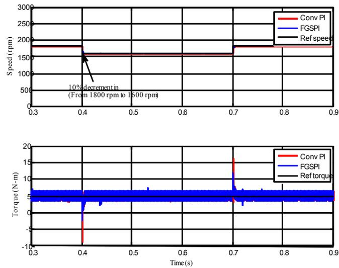
Fig. 13: Output voltage and current response of HEV system speed and torque (N=1800 rpm, T=5N-m)
