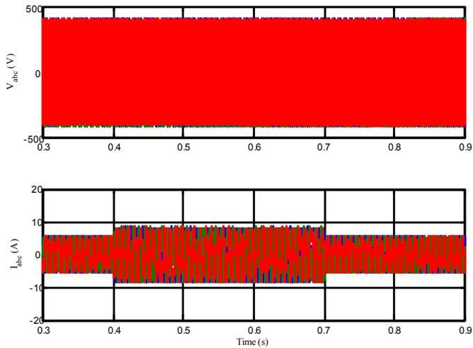
Fig. 18: Voltage and current responses of HEV system for change in load (up to 0.4sec,  $T=5\text{N-m}$ ,  $N=1800\text{ rpm}$ ;  $t= 0.4 - 0.7\text{sec}$ ,  $T=8\text{ N-m}$ ,  $N=1800\text{ rpm}$ ;  $t= 0.7 - 1\text{sec}$ ,  $T=5\text{ N-m}$ ,  $N=1800\text{ rpm}$ )
