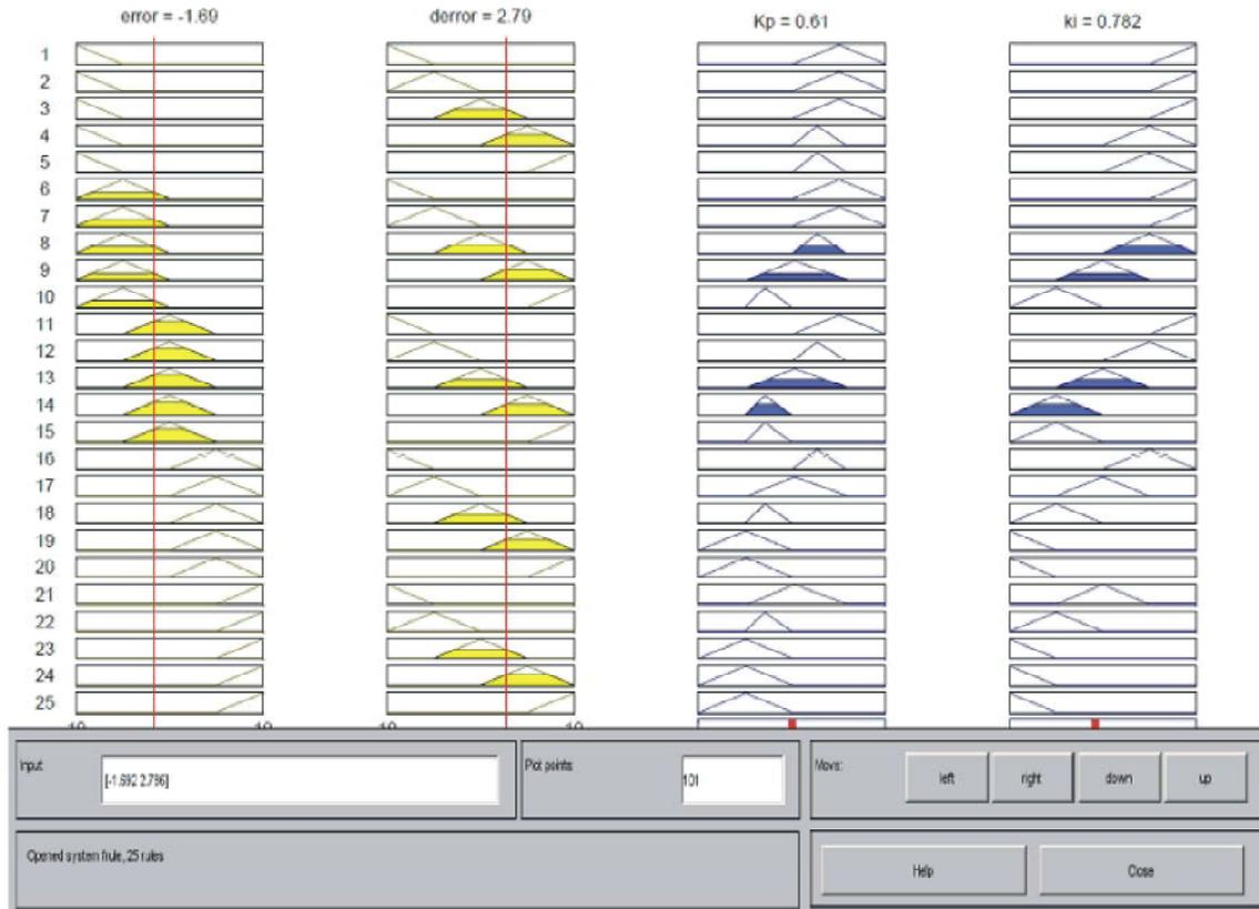
Fig. 8: Fuzzy rule base response over error, change in error and gains
