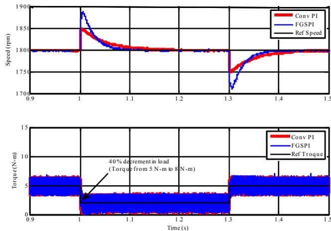
Fig. 19: Speed and torque responses of HEV system for change in load (up to 1.0sec,  $T=5\text{N-m}$ ,  $N=1800\text{ rpm}$ ;  $t= 1.0 - 1.3\text{sec}$ ,  $T=2\text{ N-m}$ ,  $N=1800\text{ rpm}$ ;  $t= 1.3 - 1.5\text{sec}$ ,  $T=5\text{ N-m}$ ,  $N=1800\text{ rpm}$ )
