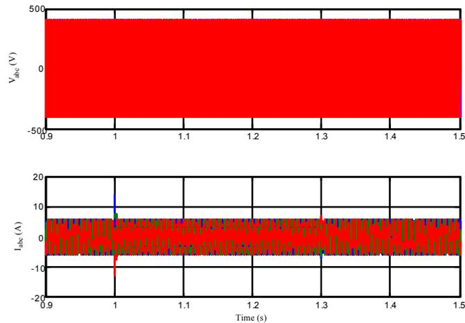
Fig. 16: Voltage and current responses of HEV system for change in speed ( $N=1800$  rpm up to 1 sec,  $T=5N\cdot m$ ;  $t=1 - 1.3$ sec,  $N=2000$  rpm,  $T=5N\cdot m$ ;  $t=1.3 - 1.5$ sec,  $N=1800$  rpm,  $T=5N\cdot m$ )
