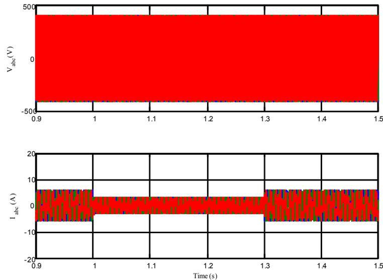
Fig. 20: Voltage and current responses of HEV system for change in load (up to 1.0sec,  $T=5\text{N}\cdot\text{m}$ ,  $N=1800\text{ rpm}$ ;  $t= 1.0 - 1.3\text{sec}$ ,  $T=2\text{ N}\cdot\text{m}$ ,  $N=1800\text{ rpm}$ ;  $t= 1.3 - 1.5\text{sec}$ ,  $T=5\text{ N}\cdot\text{m}$ ,  $N=1800\text{ rpm}$ )
