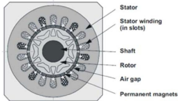
Fig. 2: BLDC Motor - Cross Section
