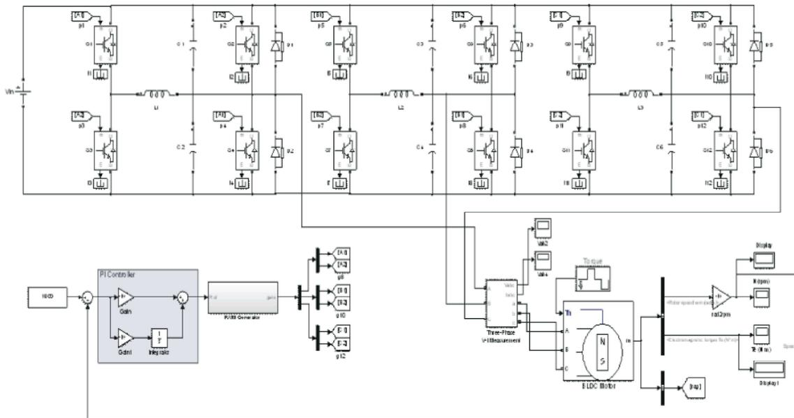
Fig. 9: Three phase resonant inverter fed HEV system using conventional PI controller
