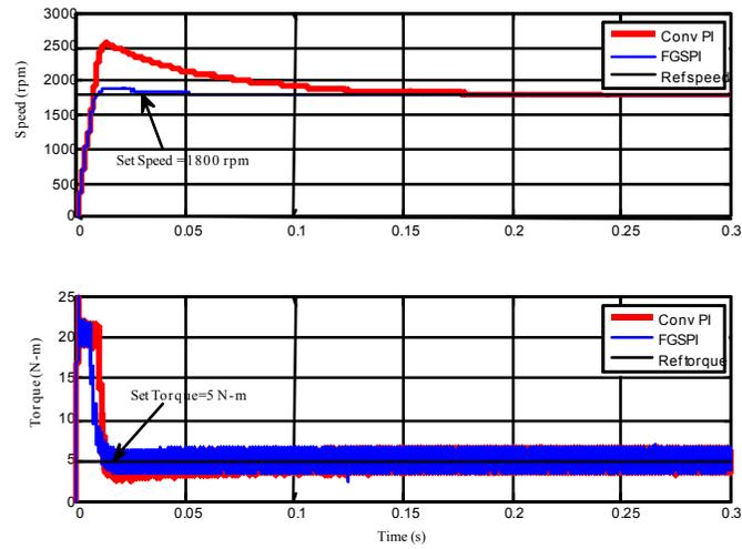
Fig. 11: Steady state response of HEV system speed and torque (N=1800 rpm, T=5N-m)
