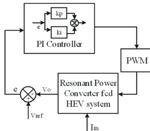
Fig. 4: Structure of PI controller with HEV system
