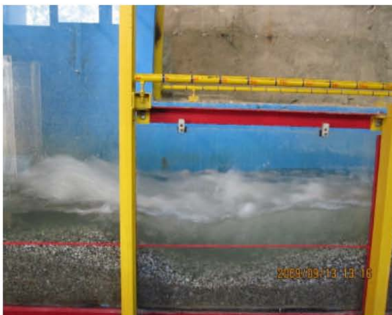
Fig. 3: A sample of scour development at the downstream of bucket
