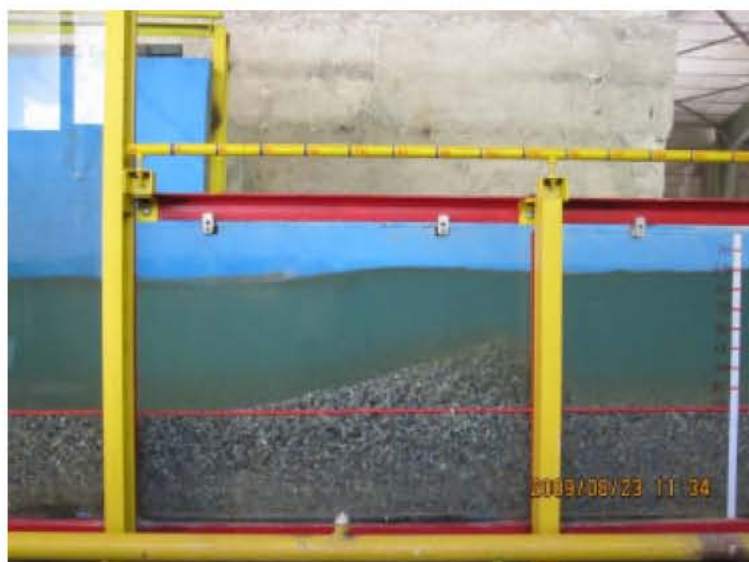
Fig. 4: Bed profile after water relaxation
