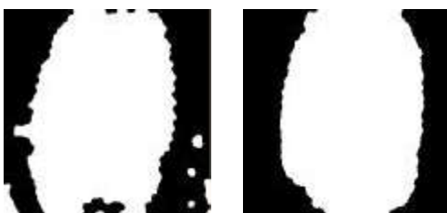
Fig. 6: The region after open operator
