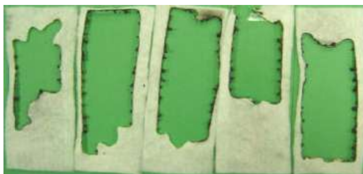
Fig. 2: Cotton blend nonwoven treated with 0.1% reactive nanosilicone softener after the flammability test
