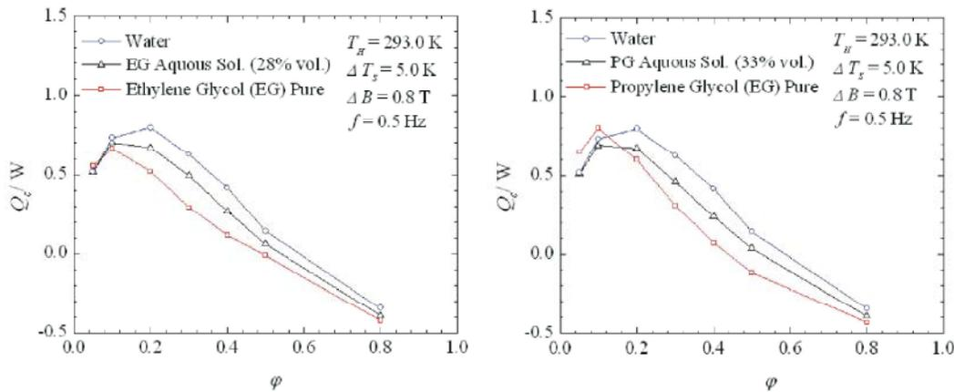
Fig. 5: Cooling power vs Utilization for water, pure glycols and their aqueous solutions
