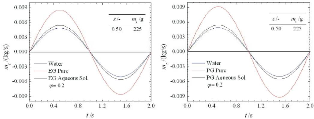
Fig. 1: Mass flow rate profiles for water, pure glycols and their aqueous solutions
