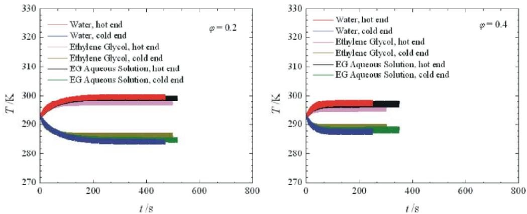
Fig. 2: No-load temperature spans for water, EG pure and EG aqueous solution at different utilizations
