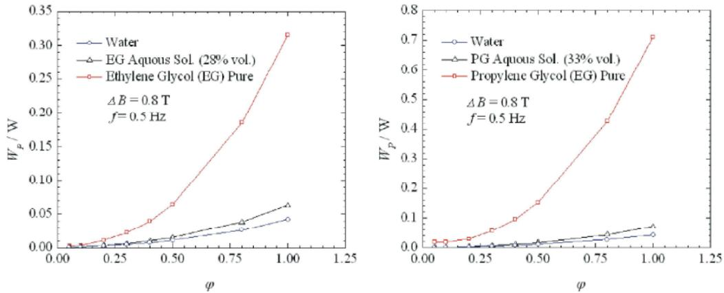
Fig. 6: Pumping power vs Utilization for water, pure glycols and their aqueous solutions
