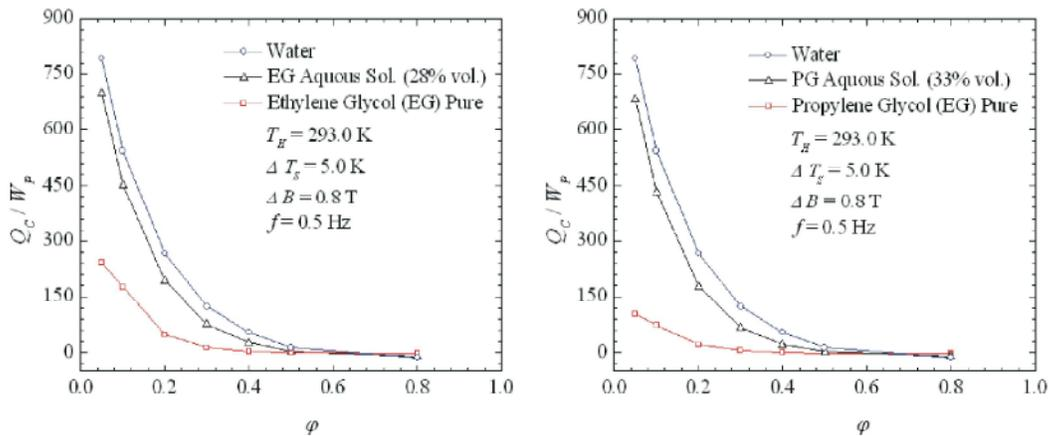
Fig. 7: Cooling capacity per unit pumping power for water, pure glycols and their aqueous solutions
