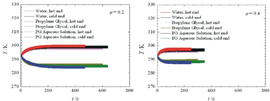
Fig. 3: No-load temperature spans for water, PG pure and PG aqueous solution at different utilizations
