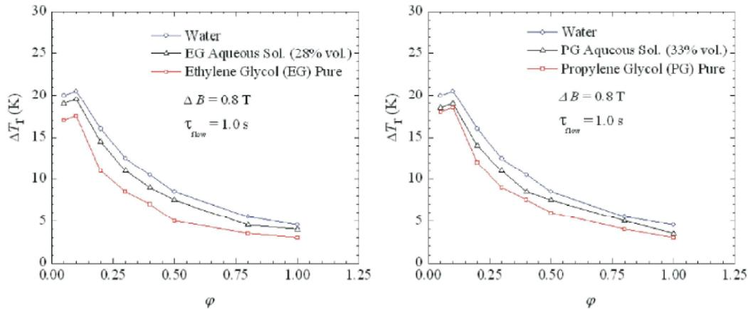
Fig. 4: Temperature span vs Utilization for water, pure glycols and their aqueous solution
