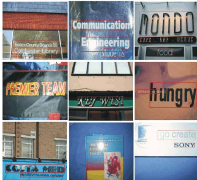
Fig. 3: Text detection examples on the ICDAR 2011 dataset. Detected text by our system are labeled using red rectangles. Notice the robustness against low contrast, complex background and font variations.
