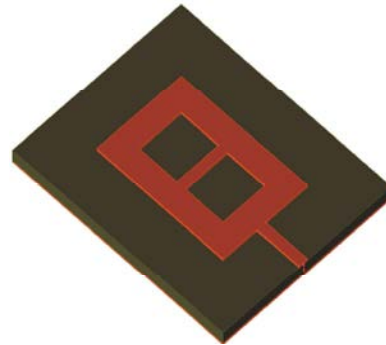
Fig. 1: Eight-Shaped Microstrip patch antenna fed by Transmission line
