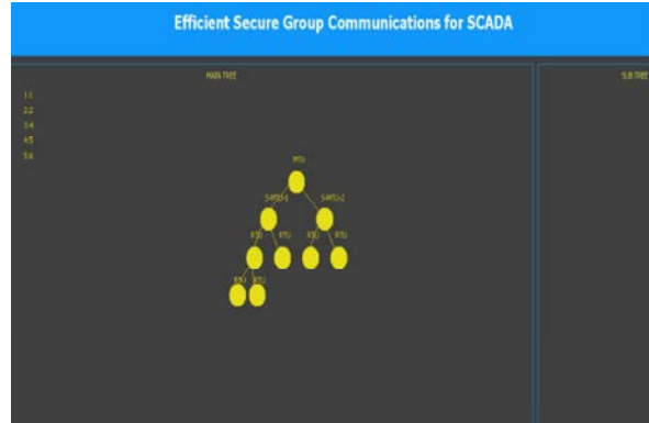
Fig 2: LKH Binary tree constructed for group members who joins and leaves the group
