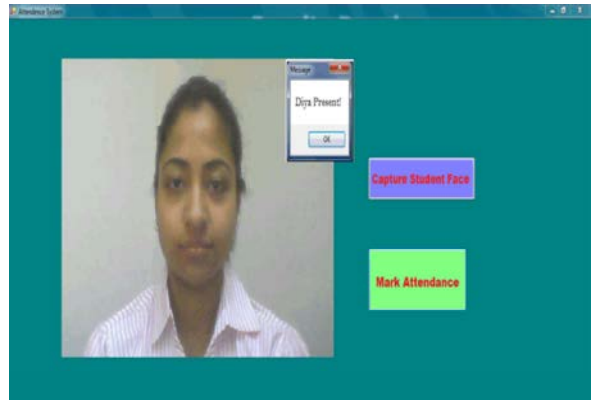
Fig. 4: Attendance of Student marked on the basis of matching real-time snapshot against database image of student
