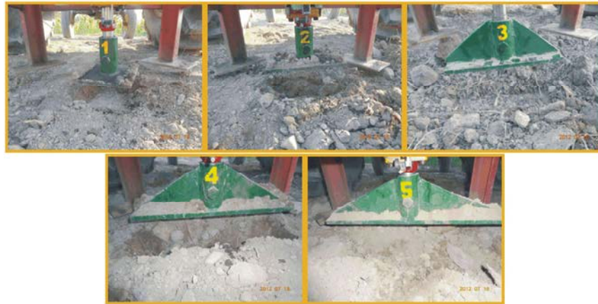
Fig. 3: Five rectangular plates used to determine soil stiffness constants in Bekker model
