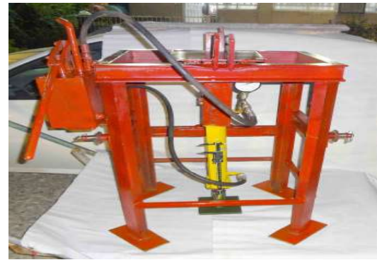
Fig. 2: Tractor mounted pressure-sinkage test apparatus
