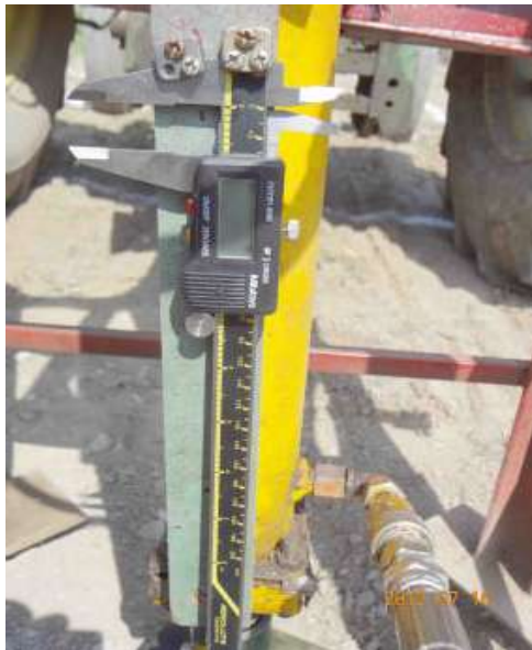
Fig. 4: A digital caliper used to measure soil sinkage
