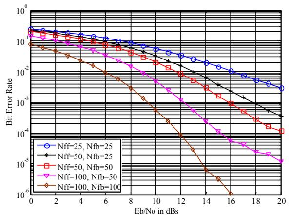
Fig. 7: BER Comparison of DWMT system for ADSL channel for different feedforward and feedback filter taps with AWGN, NEXT and FEXT
