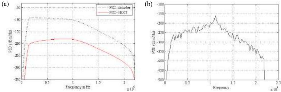
Fig. 5: (a) PSD-disturber & PSD-NEXT for downstream ADSL in G.992.1/G.992.2 standard (b) PSD-FEXT for downstream ADSL in G.992.1/G.992.2 standard.
