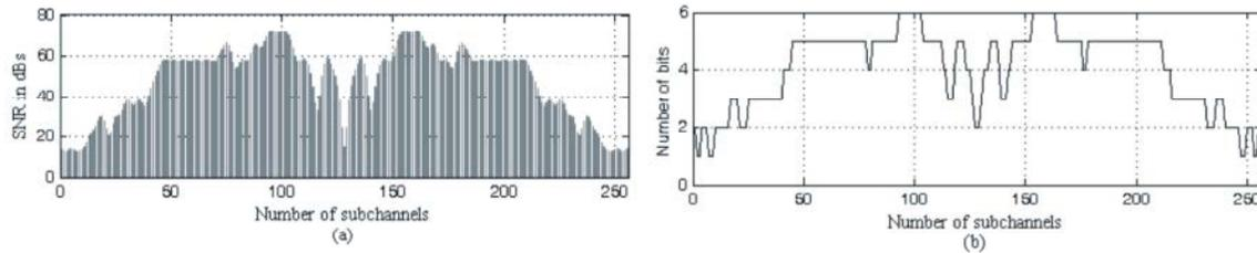
Fig. 2: ADSL channel frequency response and number of bits loaded according to discrete water-filling bit-loading algorithm.
