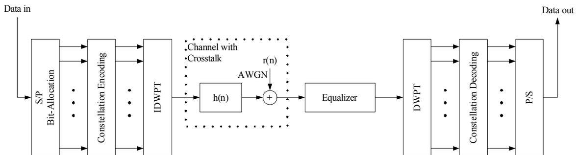
Fig. 1: Functional Block diagram of DWMT system.
