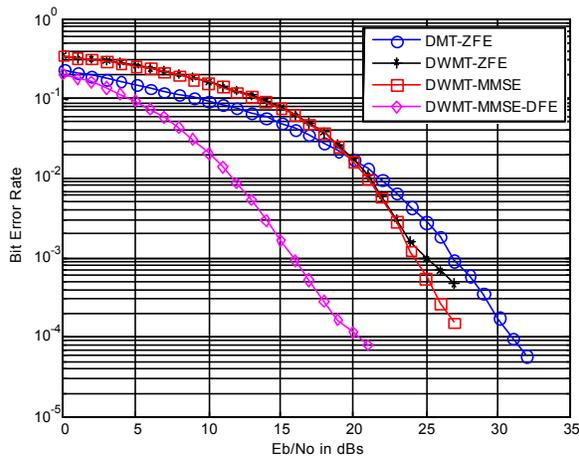
Fig. 6: BER Comparison of DWMT and DMT systems for ADSL channel with AWGN, NEXT and FEXT (Nff = 50, Nfb = 50 for MMSE-DFE)
