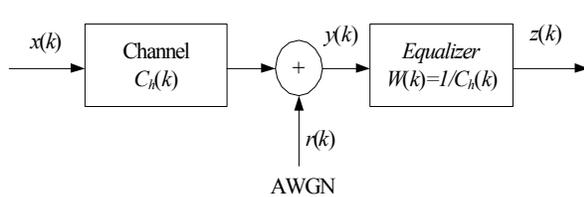
Fig. 3: A Linear transversal equalizer with coefficients optimized by Zero-Forcing criterion.
