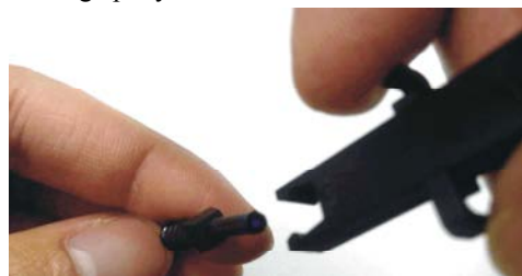
Fig. 2: Plug assembly attached with thin-film is secured by inserting the edge inside bulkhead receptacle
