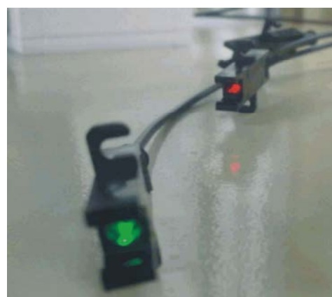
Fig. 4: Both red and green LED sources are injected to both red and green thin-film respectively
