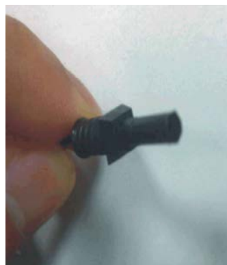
Fig. 1: Thin-film attached to the plug assembly or socket using epoxy-resin
