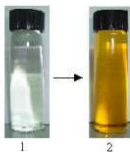
Fig. 5: Color changes of BDABD (1.0 × 10 -5 M) in acetone upon addition of Cu 2+ ions.
