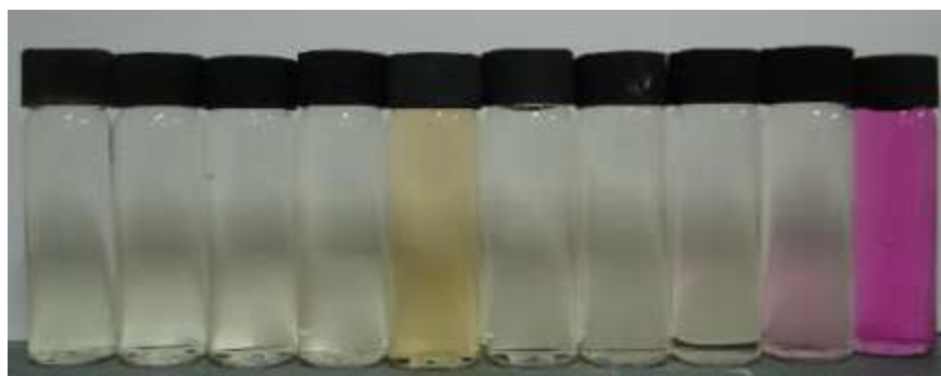
Fig. 2: Color changes of BDABD ( 1.0 \times 10^{-5} M) in ACN upon addition of various metal ions. From left to right: addition of \text{Li}^+ , \text{Na}^+ , \text{Mg}^{2+} , \text{Ca}^{2+} , \text{Zn}^{2+} , \text{Ag}^+ , \text{Pb}^{2+} , \text{Ni}^{2+} , \text{Cd}^{2+} and \text{Cu}^{2+} .
