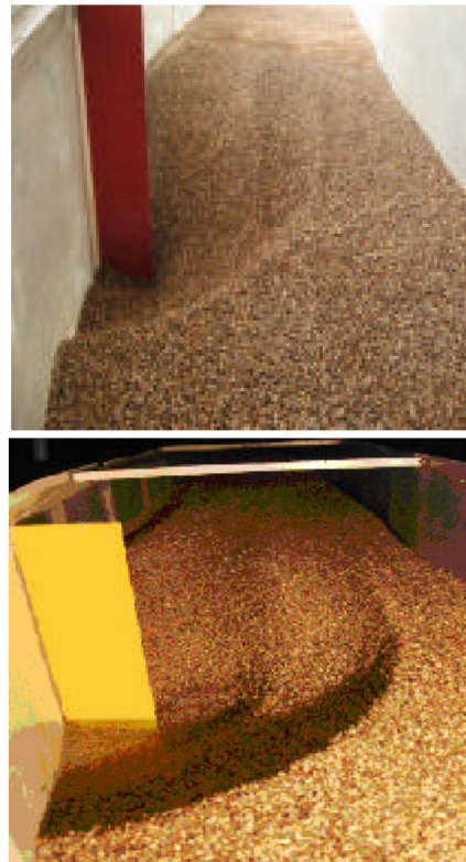
Fig. 3: Prolapse and sedimentation in the upstream and downstream of groin with lengths of 8 and 10 cm, in 170-degree position
