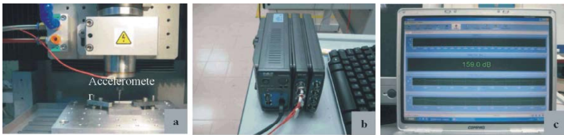
Fig. 1: Experimental setup (a) position of accelerometer, (b) multi-channel orchestra system and (c) vibration monitor with Metravib software.
