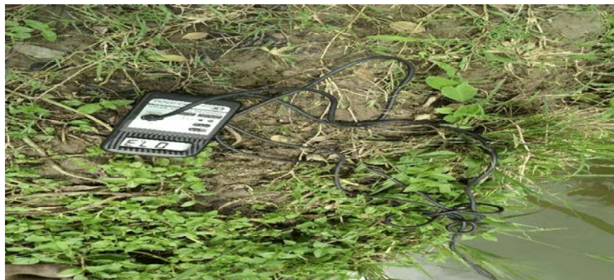
Fig. A19: Measurement of DO in experimental water body
