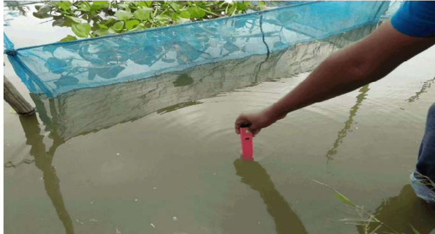
Fig. A18: pH Measurement of experimental water body
