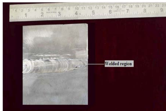
Fig. 4: Magnesium samples joined after FSW.
