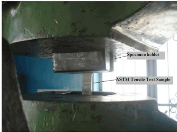
Fig. 6: Tensile specimen clamped in Universal testing machine
