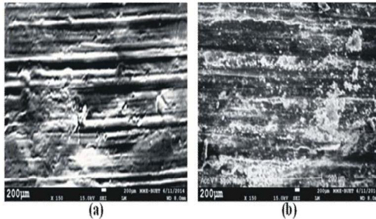
Fig. 6: SEM micrographs of the worn samples [Magnification: 150X] (a) Pure Al (unreinforced), (b) Composite (Al + 9 wt% SiC<sub>p</sub>) subjected to wear test with applied load of 20 N at 750 rpm for 10 minutes
