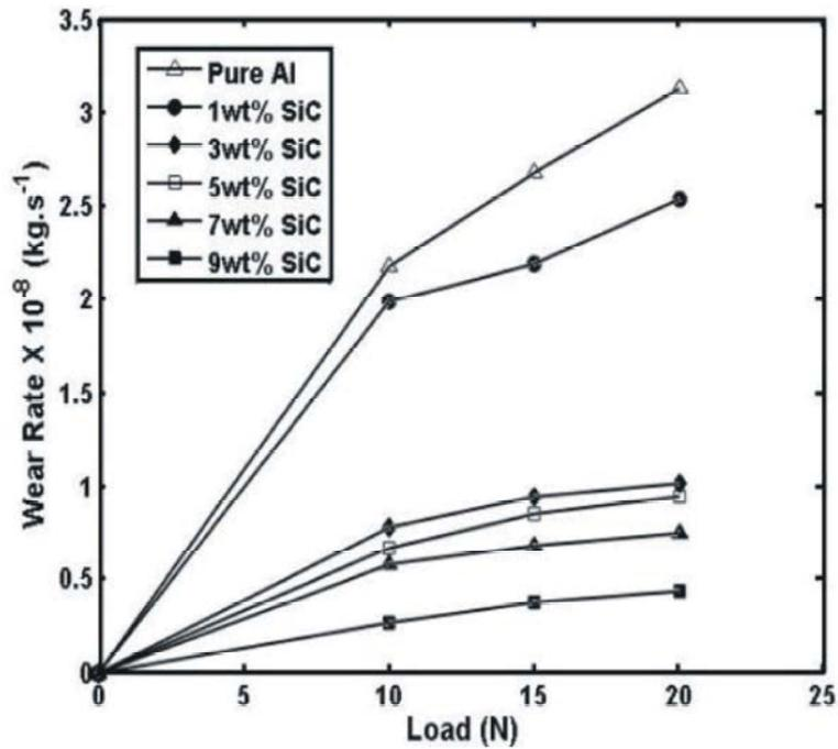
Fig. 4: Wear rate of composites with different SiC additions as a function of load
