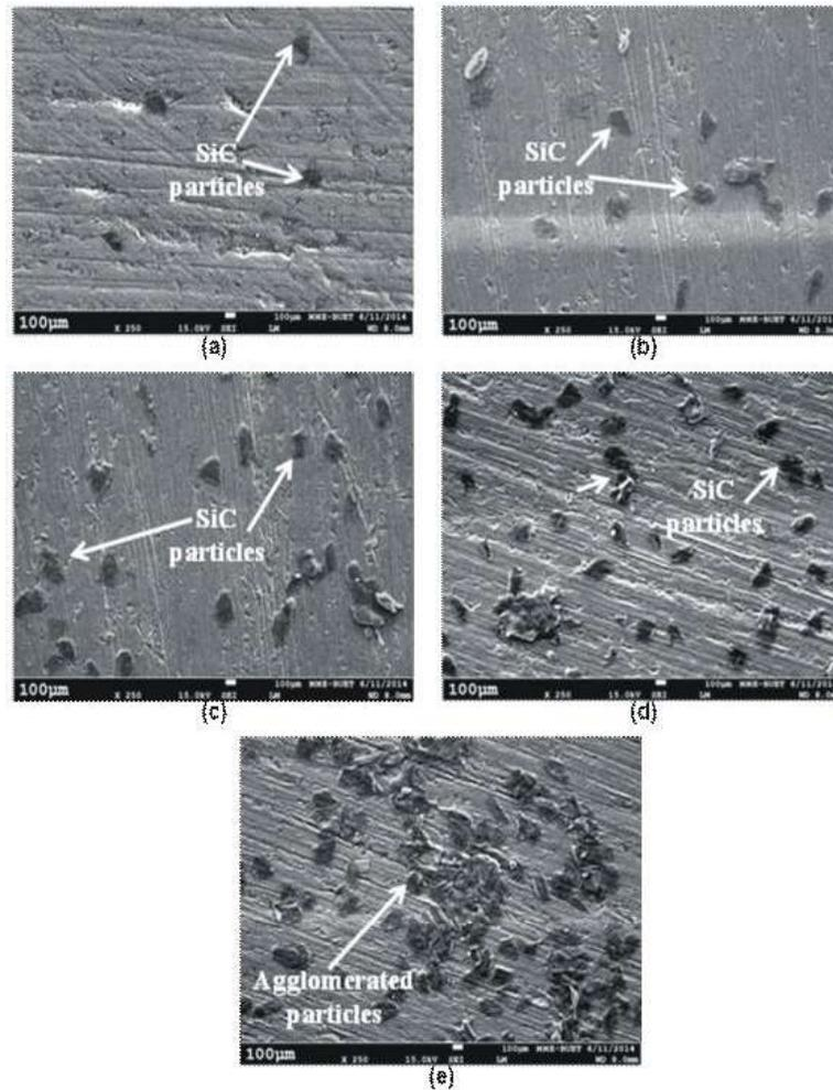
Fig. 3: Microstructure [Magnification: 250X] of composite with (a) 1 wt% SiC<sub>p</sub>, (b) 3 wt% SiC<sub>p</sub>, (c) 5 wt% SiC<sub>p</sub>, (d) 7 wt% SiC<sub>p</sub> and (e) 9 wt% SiC<sub>p</sub> in the unetched condition
