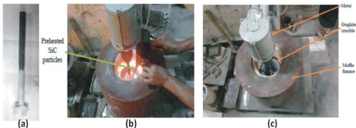
Fig. 2: (a) Graphite stirrer, (b) Addition of SiC particles into the melt, (c) Stir casting setup
