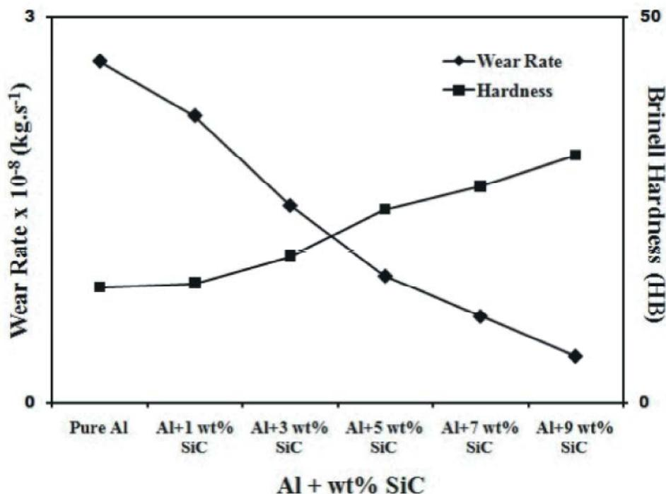
Fig. 7: Dependence of Wear Rate and Hardness on Reinforcement with SiC
