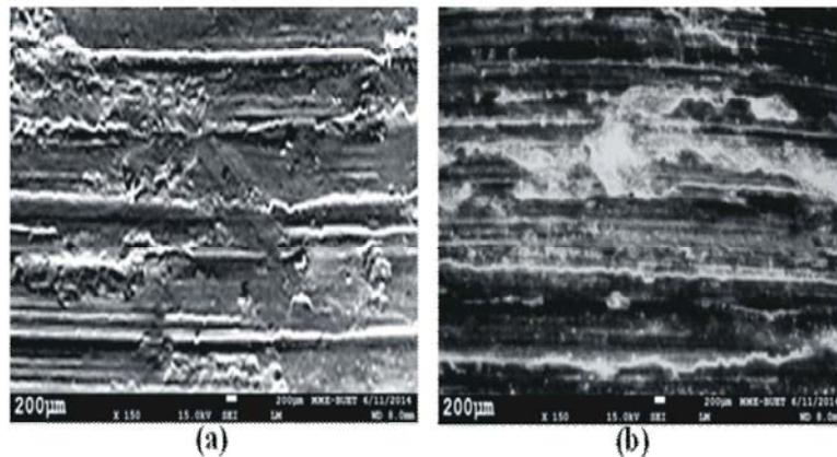
Fig. 7: SEM micrographs of the worn samples [Magnification: 150X] (a) Pure Al (unreinforced), (b) Composite (Al + 9 wt% SiC<sub>p</sub>) subjected to wear test with applied load of 20 N at 850 rpm for 10 minutes
