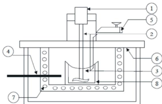
Fig. 1: Schematic view of setup for fabrication of composite (1) Motor, (2) Shaft, (3) Molten aluminium, (4) Thermocouple, (5) Particle injection chamber, (6) Insulation hard board, (7) Furnace, (8) Graphite crucible [14]
