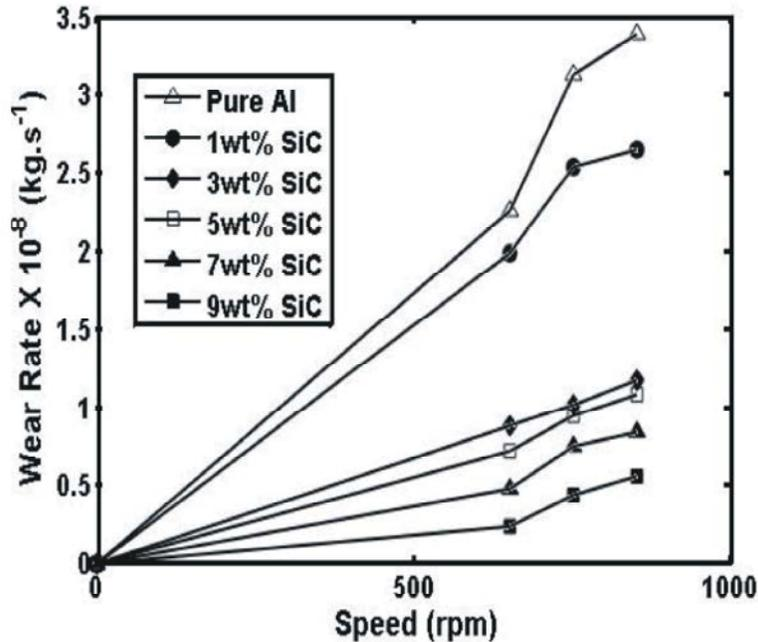
Fig. 5: Wear rate of composites with different SiC additions as a function of sliding speed
