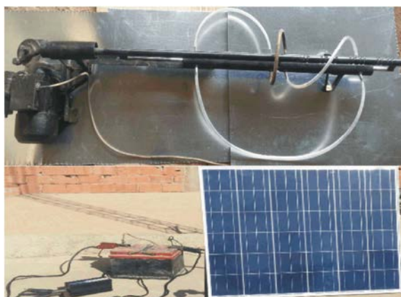
Fig. 7: Pump conception and electric conversion
