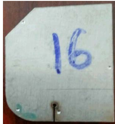
Fig. 2: Stainless steel workpiece after laser cutting
