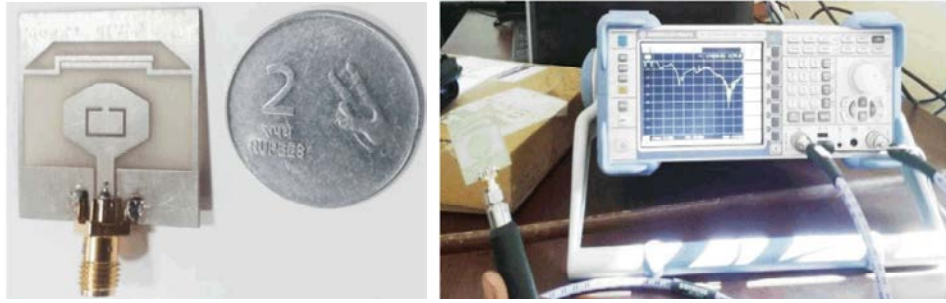
Fig. 5: Photograph of the fabricated prototype and its measurement set up
