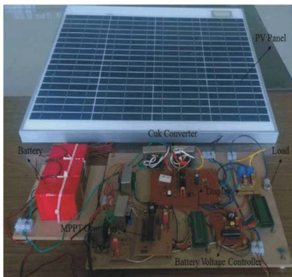
Fig. 12: Hardware setup for Cuk Converter based solar PV system for standalone system
